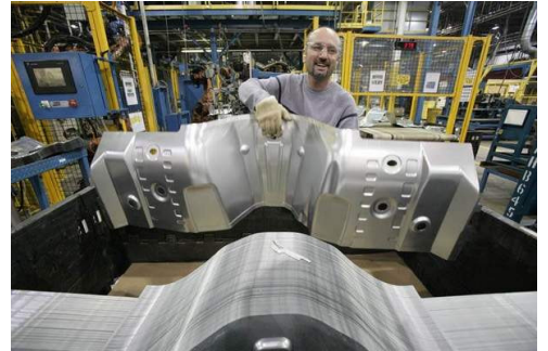
Team Associate Sami Youanes, 45, of Sterling Heights moves a front floor pan extension (for use in the Chevy Camaro) at the AZ Automotive Corp. Center Line Plant on Thursday, Oct. 29, 2009. (PATRICIA BECK/DFP)
