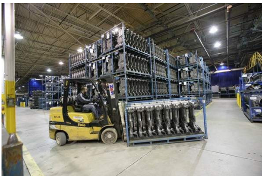
A rack of front cross-members for use on the Dodge and Chrysler Minivan, Dodge Journey, and Chrysler Sebring are moved with a fork lift at the AZ Automotive Corp. Sterling Heights Plant on Thursday, Oct. 29, 2009. (PATRICIA BECK/DFP)
